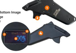
To access the menu, with the controller on, hold Trigger 3 "Cruise Control" and single press the Power Button. Once in the menu, release Trigger 3. Single (short) press the power button to scroll through the menu, press power button for 3 seconds to select.
